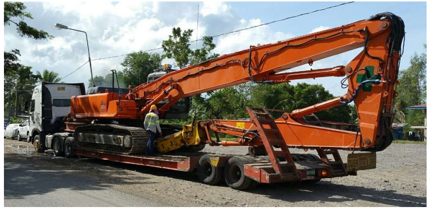
HITACHI 350LCK, WITH GENESIS 255 SHEARER/22METER LONG ARM
