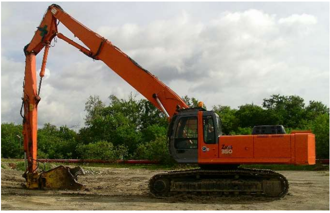
HITACHI 350LCK, WITH GENESIS 255 SHEARER/22METER LONG ARM
